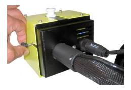
Push in sample pipe and tighten union nut stalwart only
