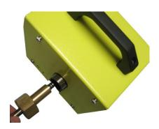
5. Mount probe gastight to sampling hole or process flange and hang JPES up with mounting chain
