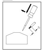
Clamp connection see the connection diagram on page 5. Cable run only through the planned PG-screwings, 2x PG9 for power / heating, 2x PG7 for sensors and signals.
