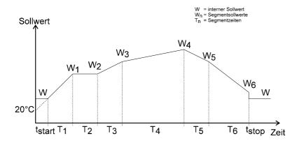
A segment- resp. program stop can be marked at alarm output Y3!
