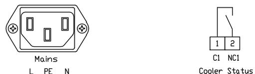
Connect to the power supply via the IEC socket.
