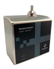
The 2510 and 2510-2 particle counters provide a range of particle size measurement from 0.5 to 5.0  $\mu$ m at a flow rate of 1.0 CFM (28.3 LPM). These sensors allow for efficient particle counting with specifications that exceed the ISO 21501-4 and JIS B9921 calibration standards.
