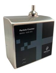
The 9301 and 9501 particle counters provide a range of particle size measurement from 0.3 or 0.5 to 10.0  $\mu$ m at a flow rate of 0.1 CFM (2.83 LPM). These sensors allow for efficient particle counting with specifications that exceed the ISO 21501-4 and JIS B9921 calibration standards.
