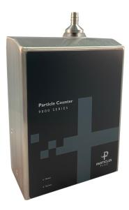
The 9301P and 9501P particle counters provide a range of particle size measurement from 0.3 to 10.0  $\mu$ m at a flow rate of 0.1 CFM (2.83 LPM). These sensors allow for efficient particle counting with specifications that exceed the ISO 21501-4 and JIS B9921 calibration standards.
