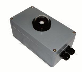
The TunnelTech 602 Illuminance photometer monitors the average illuminance within a tunnel in accordance with Commission Internationale de l'Eclairage, (C.I.E.), publication 88, 2004 recommendations, the photometer monitors the average illuminance over a range of 0 - 20,000 lux.
