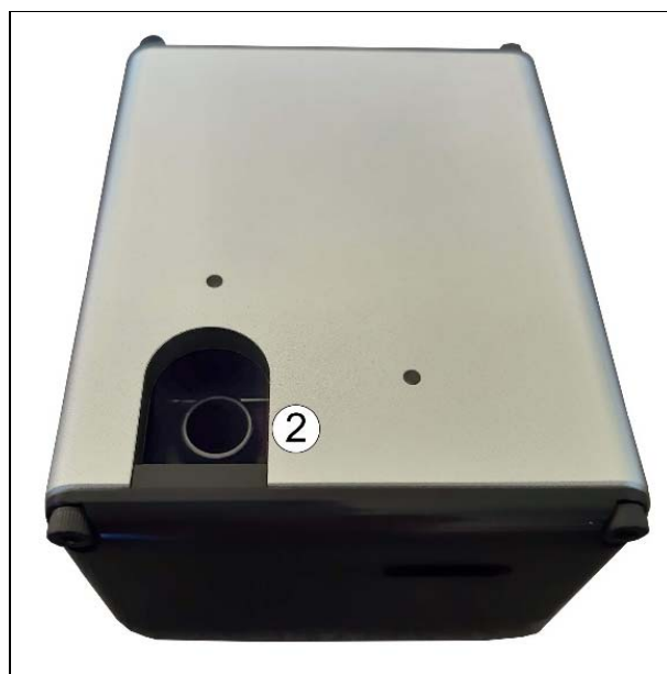
Figure 1-4 – Sample inlet view (2)
