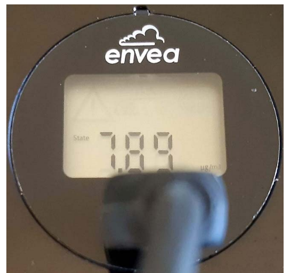
(1) Measured value displayed on three XXX digits, (2) « y » value in the formula: XXX \times 10^y
