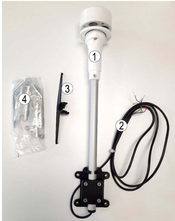
(1) Anemometer, (2) cable, (3) alignment sight, (4) fixation system on mast
